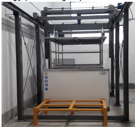
System wannowy do strippingu
