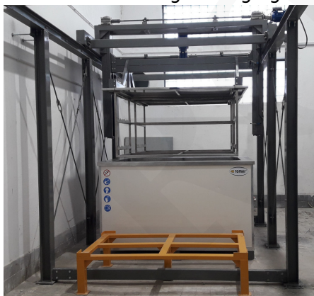
System wannowy do strippingu
